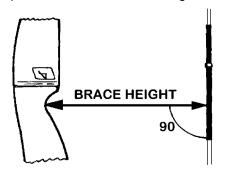
Bow manufacturers recommend a brace height for each model and length of bow, but as a guide most bows fit within the following tolerances in brace height.
