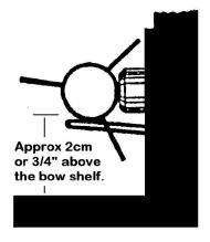
The arrow rest must be positioned correctly to ensure the arrow sits on the arrow rest square to the plunger button, this ensures even side pressure against the plunger upon release.
