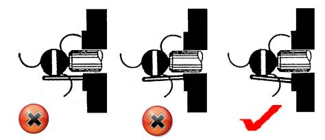
It is also important that a minimum amount of arrow rest arm protrudes out from the arrow; excess arrow arm may cause a clearance problem as the arrow moves forward.
