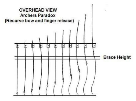
Most bows are fitted with a plunger button which is designed to initially absorb this side pressure allowing the arrow to move into centreshot as it commences its forward movement.
