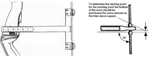
There are two common types of nocking points used. A commercially available product called "Nok Sets" and a tie on type that only requires a length of bowstring serving material. Nok Sets are great for setting up the bow as they are easy to adjust but should not be used permanently, always us the tie on type of nocking points.
