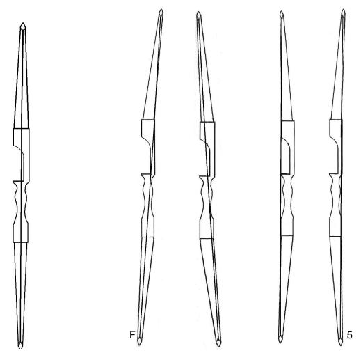
It is very important that limbs are aligned straight and that both limbs are aligned with the centre of the grip.
