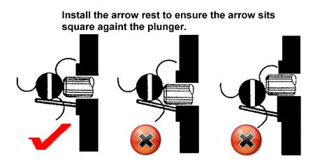
The arrow rest must also be positioned to ensure the arrow remains on the rest upon release and does not fall off the rest.
