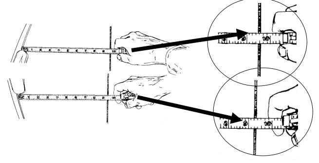
To set the tiller, firstly set the bow weight to the mid setting and then check the tiller measurement as shown above, remember we want the top limb measurement to be greater then the bottom limb.
